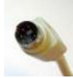
A201902 Cable RS-232 Wincor Beetle POS, Sub-D 9-pin Male DP (+EP) \*
