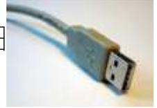
Note: The Sirius-USB must be directly connected to the PC-USB port and not through an (un-powered) USB hub.
