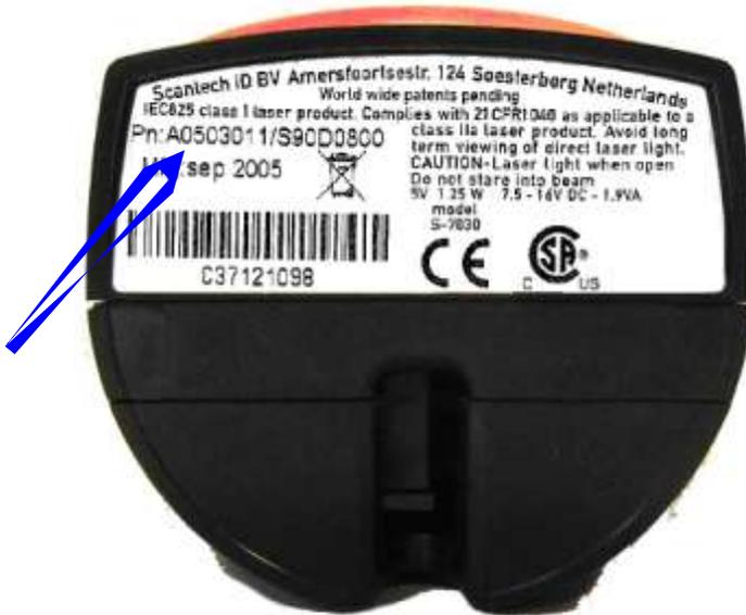
The scanner's serial number and type number are found underneath the scanner as depicted in the figure above. This official registration number is strictly related to the device. The supplier may ask for these numbers when the scanner needs servicing.
