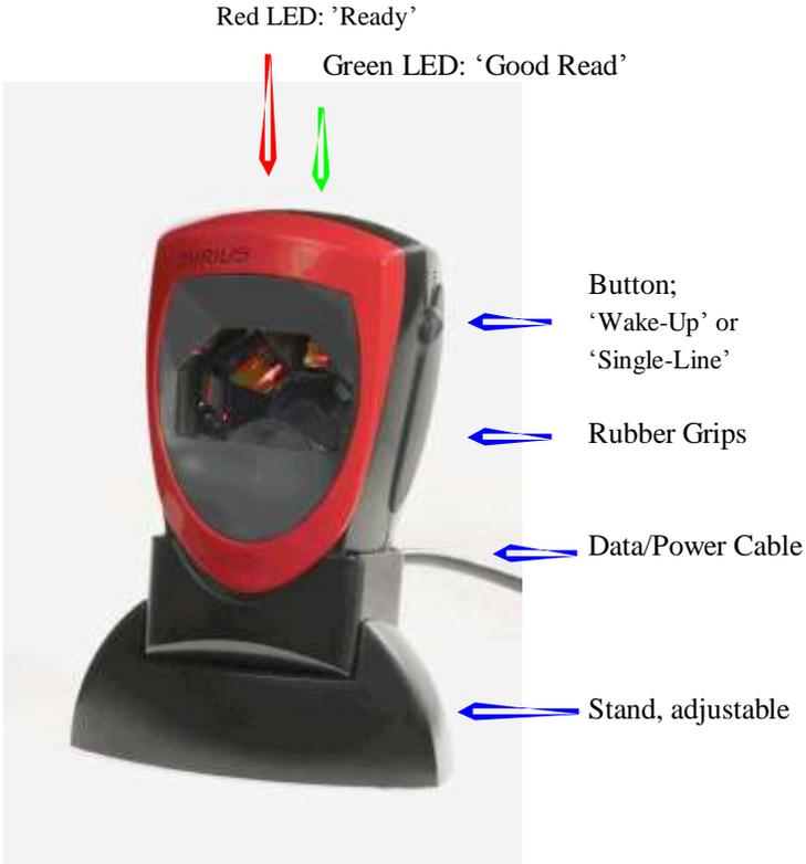
Adjust the orientation of the scanner the scanner by rocking it carefully while mounted in the stand and by rotating the stand on its floor surface.
